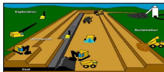
Gambar 3.3 Skema Penambangan Open Pit Mining
