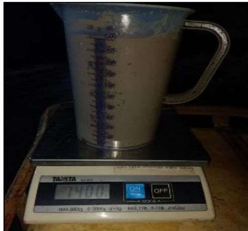
Gambar 3.5 Perhitungan SG Sump Pit Z
